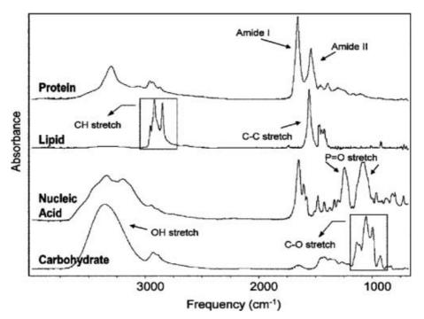
Fig. 1 – Infrared spectra for different cellular components.
