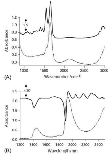
Fig. 2 – Mid-infrared (a) and near-infrared (b) absorption spectra of serum (dashed lines) and the residual spectra with the spectrum of water subtracted from each (solid lines).
