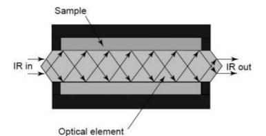
Fig. 3 – Apparatus to measure the ATR spectrum for a liquid specimen.
